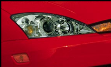
High-intensity discharge headlamps are available on the SVT Focus
