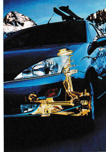
MacPherson struts remain up front
