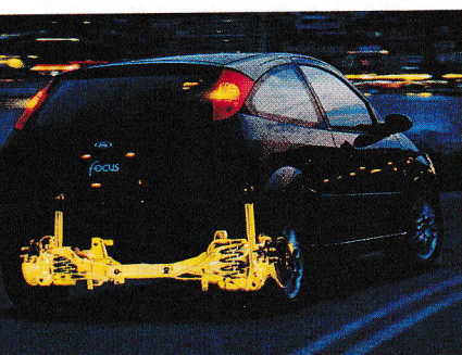
New multi-link rear suspension helps to give class-leading ride, says Ford
