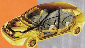
All three rear seat passengers are provided with lap and diagonal inertia-rear seat belts. Picture below includes optional centre rear head restraint. For further information about Ford child safety seats please ask your main Ford Dealer.
