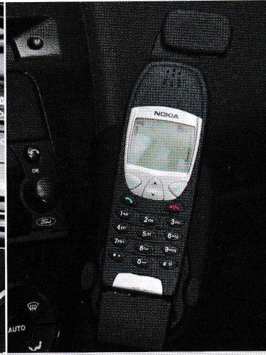
Nokia compatible hands-free mobile phone kit option consists of a telephone console, cradle, base kit, antenna and microphone*. Compatible with Nokia 5110, 5130, 6150, 6110, 6130, 6210, 6310, 6310i only.
