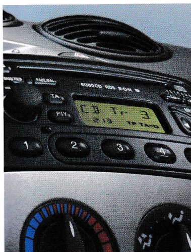
Model 6000N RDS EON with remote column-mounted controls, removable control panel, 'Keycode' anti-theft coding, 4 speakers.
