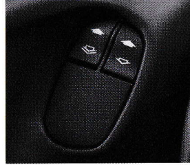
Electric front windows feature one-shot lowering on the driver's side.
