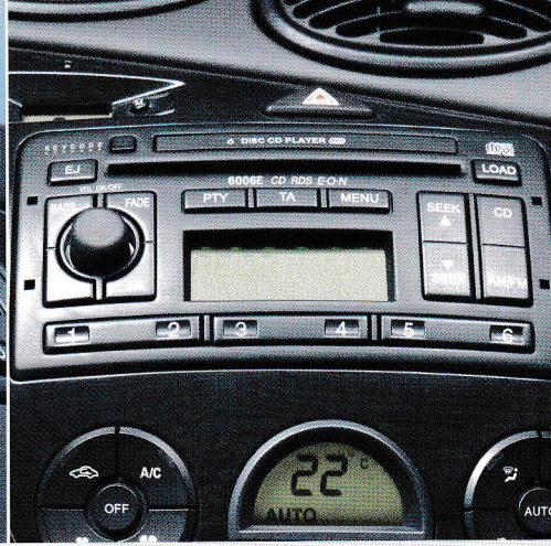
Model 6006 RDS/EON radio/CD player – four-channel AM/FM radio with 24 presets, electronic search facilities and a 6-disc CD autochanger. Peak output is 4 x 48 watts.
