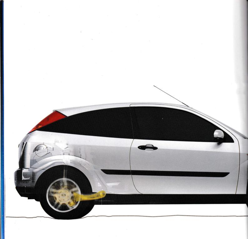
The key to the Focus' suspension system is the unique Control Blade system to deliver precise control and superior comfort. The control blade is a light, yet strong, one-piece pressed steel component providing greatly improved stability and active safety – even in the most extreme driving conditions.
